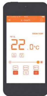
The e-touch® control system is a fully portable, rechargeable, blue-tooth based touch screen unit, featuring a built-in thermostat, enabling you to regulate and maintain the selected room temperature with ease.
